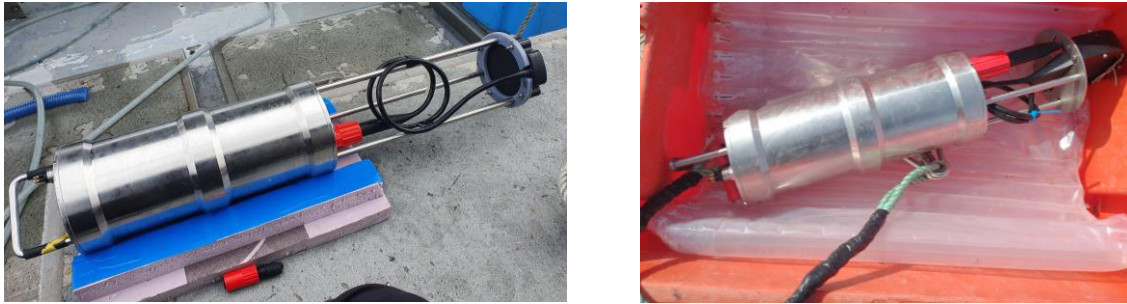
Figure 1. The TAST prototype (GenusWave Ltd), versions 1 (left) and 2 (right, with improved ergonomic design based on feedback from fishers to engineers at GenusWave Ltd), used in trials. The watertight housing (stainless steel) measures ~60 cm in length and ~20 cm in diameter, with a total weight of water of around 12 kg. It is pressure compensated and suitable for deployments down to around 100 m depth.
